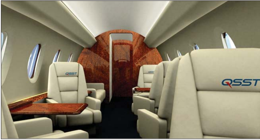
SAI's QSST is designed to carry up to 12 passengers in large-cabin comfort, including more than 6 ft of headroom, a galley and full lavatory, and access to baggage during flight.
